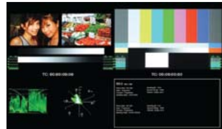
Dual 3 Gb/s Input Display Mode SDI-1, SDI-2, Waveform / Vectorscope, 16 CH Audio Level Meter, VPID & Time Code
