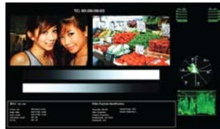
Waveform + Vector Scope + VPID SDI-1, Waveform / Vectorscope, 16 CH Audio Level Meter, VPID & Time Code
